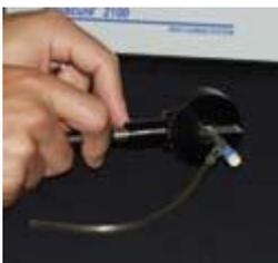
Cure rings enable a 360° cure and can be fixed (above) or hinged.
