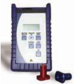
A handheld radiometer is similar in size to a personal digital assistant and enables the user to set all systems remotely..
